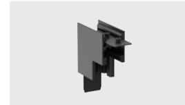
L-shaped(Inward) Model: MT11-L90N-MH11 Material: Aluminum Size: L39.5×W39.5×H19mm Applicable model: TLS-MT11-HXO
