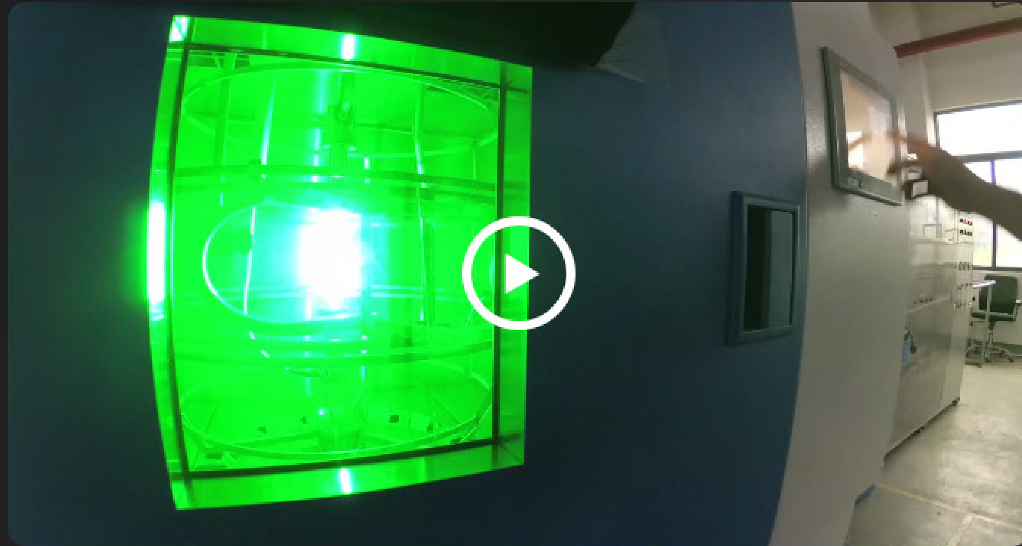
High-intensity 3000 Hours UV Test Equivalent to 9 years of outdoor use almost no yellowing
